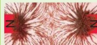
▲ Magnets with like poles facing each other
